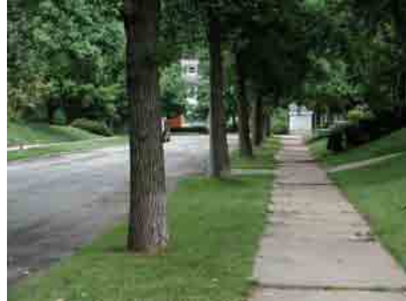
6.3.5 Tree Lawn. A tree lawn is a continuous landscaped strip between the edge of a street and a detached sidewalk.
